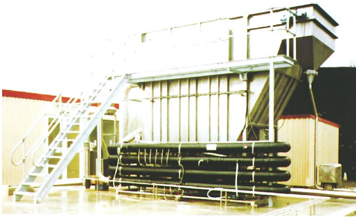
Fig. 3 Flotation system, type KCL 120, capacity 300 m 3 /hr., including pipe flocculator
